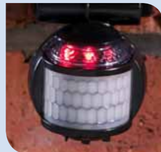
MLB3000/MLW3000 Scrolling LED 'System Live' status indicator.
